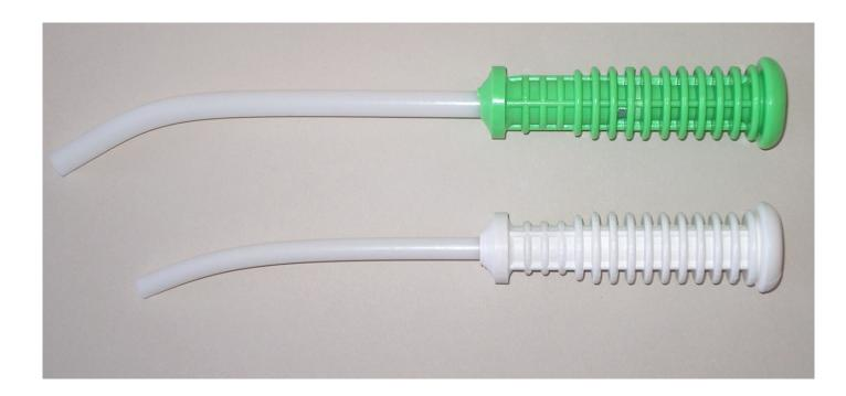
For the best results when packing a stuffing box, each packing ring should b tamped firmly into place to insure a seal to the shaft and the walls of the stuffing box. These tools are designed to help you accomplish that.
