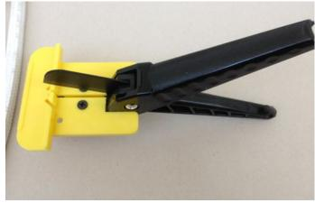
The spring loaded adjustable quide fence locks into 90 and 45 degree positions for fast accurate cuts every time. To change guide fence position- just lift and turn. Max dimension of 90° cut = 25x25mm / of 45° cut 16x16mm.
